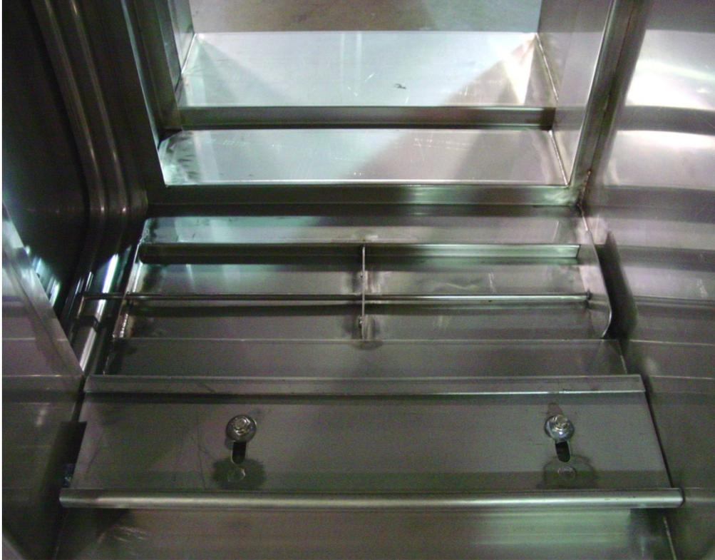
(downstream view of locking tray mechanism)
